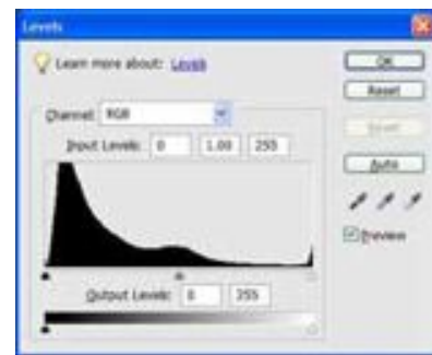
Although most pixels are toward the dark side, the small area clipped on the right indicates a blown out highlight.
